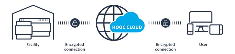
Remote access with EIBPORT V3 and CUBEVISION or APP MODULE is as simple as can be: Thanks to the integrated VPN solution, there's no need to purchase and install costly additional hardware anymore.
